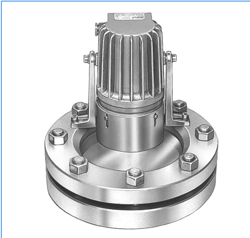
VETROLUX illuminated sightglass unit, consisting of sightglass to DIN 28120, DN 150, PN 10, with mounted CHEMLUX light fitting, type KEL 20 deH Sch B, 230 V, 20 W, Ex d e IIC T4 Gb, Ex t IIIC T130°C Db IP67, Ex II 2 G + D, with anti-dazzle shield "B", in version "view and light through one assembly"
