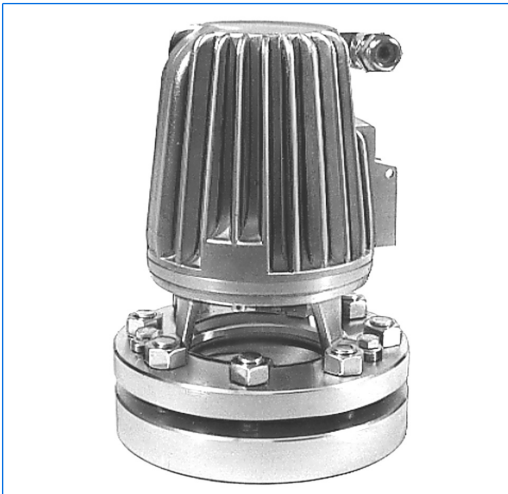
VETROLUX illuminated sightglass unit, consisting of sightglass to DIN 28120, DN 80, PN 10, with mounted CHEMLUX light fitting, type F 20dHNsp, 24 V, 20 W, Ex d IIC T5 Gb, Ex t IIIC T95°C Db IP 67, Ex II 2 G + D
